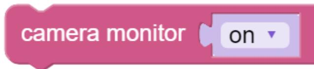
This block is used to enable the camera module.
