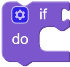
We used an **if** block (you can find it in the **Logic** category on the left) to make the PiCrawler move forward once when the **UP** button of the D-pad is pressed.
