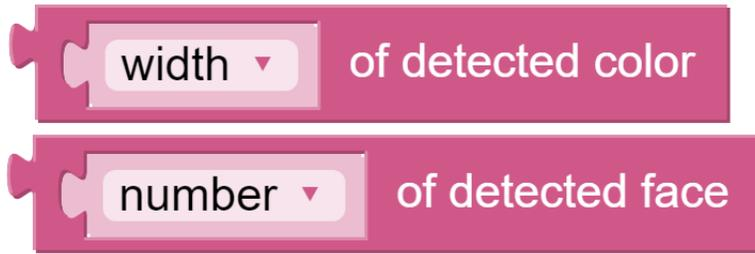
These two blocks are used to output information. The detection result has five output values, namely coordinate x value, coordinate y value, width, height, and number.
